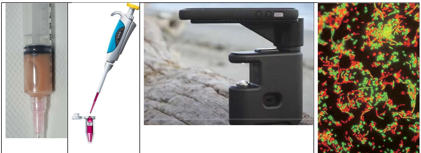
Figure 3 – real example of our technique. Joint aspirate is performed followed by addition of bacterial-specific dyes and then viewed under a portable microscope (insignificant cost) with a real example image on the right.
